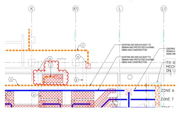
2.2 Existing 300x200 E/A duct routing is updated as shown clouded. The location of existing E/A duct up to existing exhaust fan on the roof is updated as shown clouded in below.
