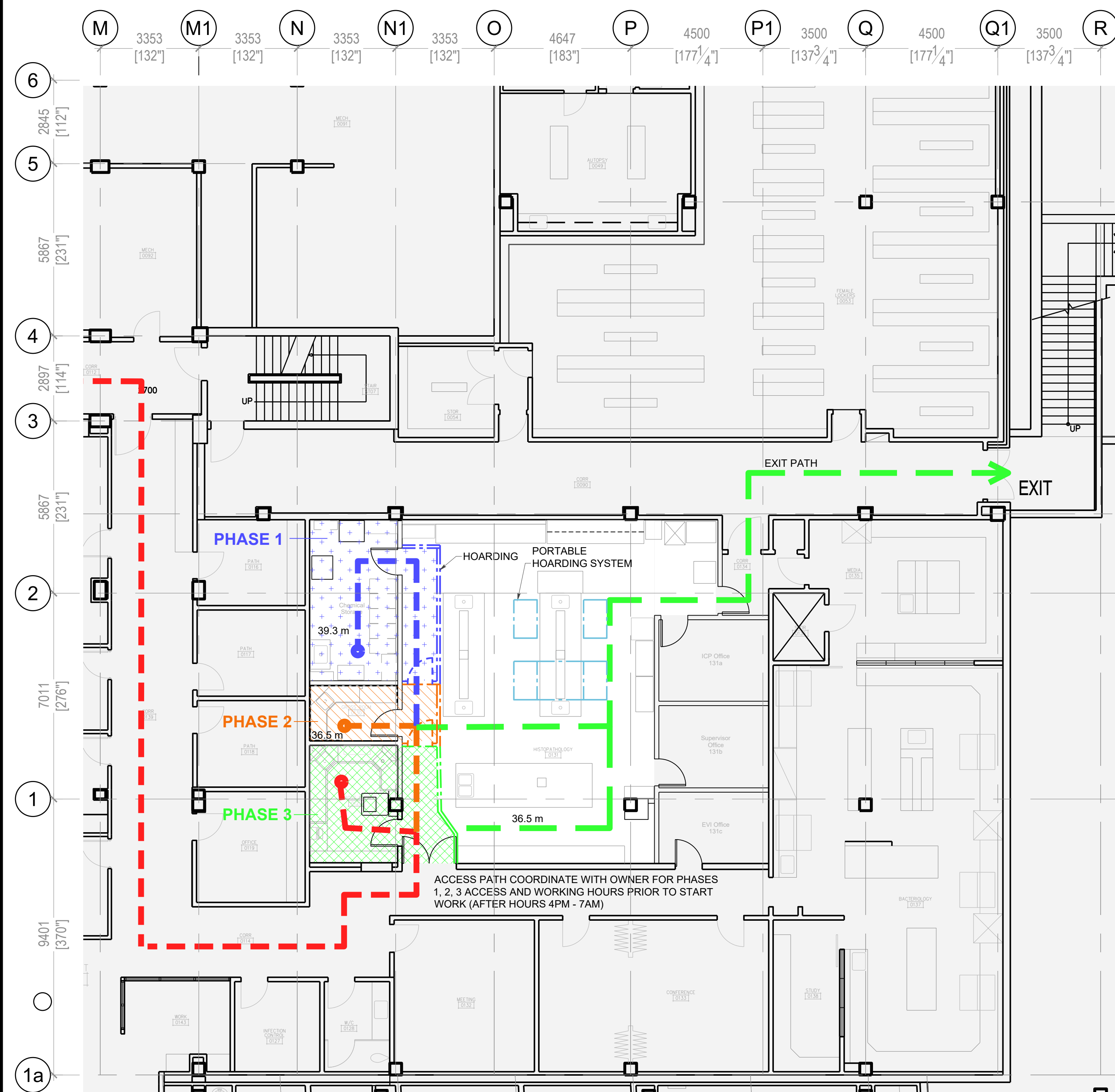
1 SAFETY PLAN & PHASING CONSTRUCTION A-100 1:100
